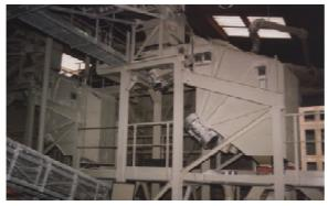
3 suitable for: selections 0.2 to 40 mm, feed size 1 to 500 mm, capacities 1 to 1200 m3/h
